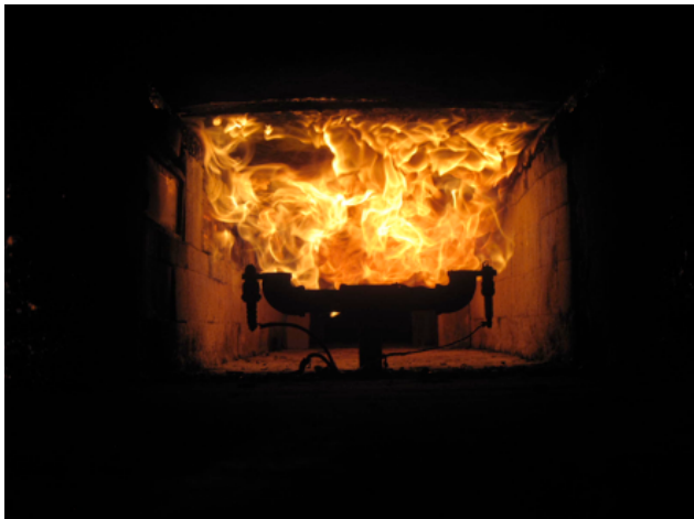
Figure 1. View of the Steiner Tunnel, showing flame being applied to the ceiling (Photo: Intertek Testing Services, Inc.)
