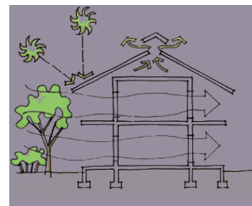
Broward County County-Wide Community Design Guidebook, Broward County Board of County Commissioners, Anthony Abbate, Architect PA. Note recommendations for climate-responsive architectural design strategies: building form with deep overhangs to promote sun shading and natural ventilation and use of trees for solar and breeze control.
