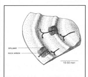
Swales, or curvilinear depressions in the earth combined with berms, can be on-contour to retain stormwater or off-contour to direct water downhill in a controlled manner.
