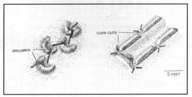
Microbasins are small basins used to retain low volumes of runoff. When used in parking lots, they can water trees that shade the pavement and cars.
