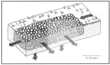
French drains are rock-filled trenches that promote water infiltration deep into the soil. They work best for runoff that has a low sediment load.
