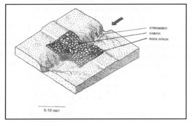
Gabions are semipermiable rock barriers constructed in small (less than 25 cfs in a 100-year flood) drainages. They slow but do not stop the flow of water and help prevent erosion, trap sediment and organic matter, and allow water to infiltrate.
